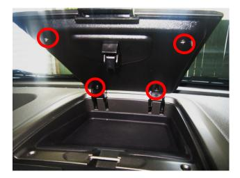
2. Remove latch assembly (3 Phillips screws):
