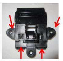
You end up with: Latch base, Latch cover, Broken latch, and 2 springs.
