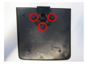
3. Pry latch assembly apart with flat bladed screwdriver. This part may be brittle—be gentle and loosen it slowly.
