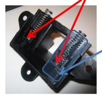
(Optional—apply a small amount of grease / WD40 to springs and where the latch slides)
